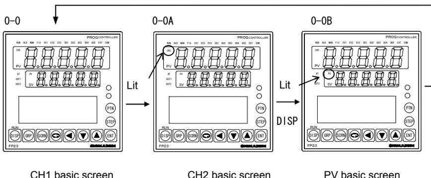
The channel display in these basic screens is interlocked with the PV display, SV display and five status indicators (RUN, HLD, MAN, FIX, EXT). The CH1 is displayed when the CH2 indicator is out, and the CH2 is displayed when the CH1 indicator is out.
