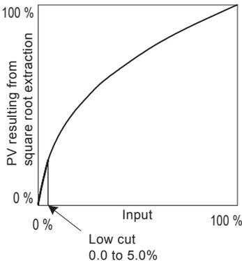
**Note** Low cut processing is performed on input, and square root extraction processing is performed.
