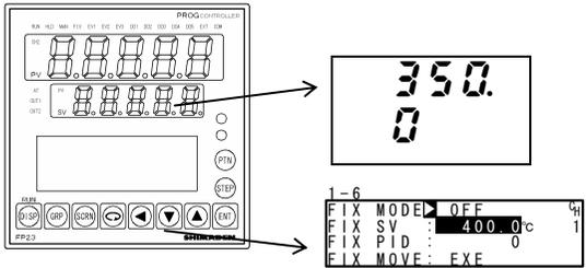
The white-inverted section indicates limit over.
