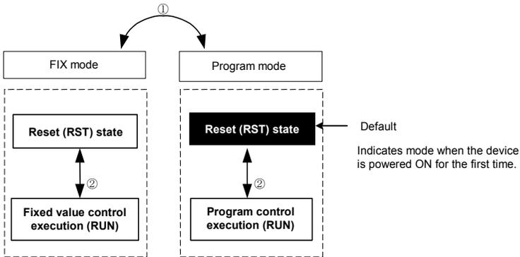
① The FIX mode is switched by the FIX mode ON/OFF settings in the FIX MODE screen (No.1 to 6). The mode switches to the FIX (fixed value) mode when ON is set, and to the program mode when OFF is set.
