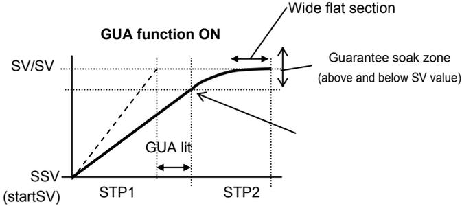
When the deviation between the step SV and PV of the flat step does not enter the guarantee soak zone when the ramp step switches to the flat step, the program does not move to the next step, and stands by until this region is reached or the GUA time ends.
