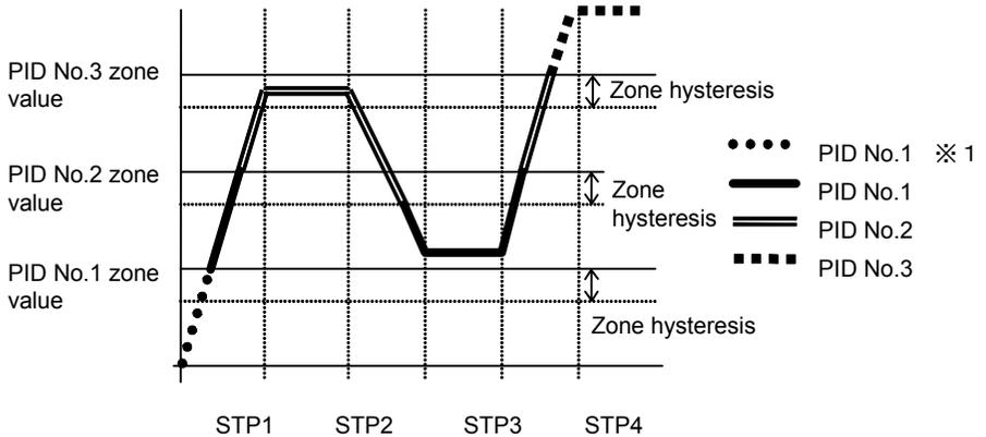
Note 1      When the same zone value is set to two or more PID Nos., the PID having the smallest No. is executed.
