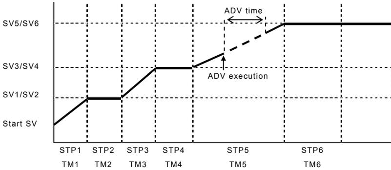
\*1 In time selection, when the ADV time is greater than the remaining time of that step, advance beyond the next step is not performed, and the program only advances to the next step in the same way as in step selection.
