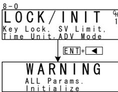
A warning is displayed on the LCD screen, and the setup parameters in the table below are displayed on the PV/SV displays.
